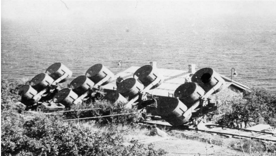
Fig. 5.6. Photograph of the Crimean multi-telescope setup. Each barrel contains one Cherenkov telescope. Three telescopes form a unit. Each of those units can be positioned along a railway system and view the air showers under slightly different angles. This arrangement allowed both coincidence measurements and simple multi-telescope observations. The system was used from 1960 until 1963. Figure courtesy T. C. Weekes.
